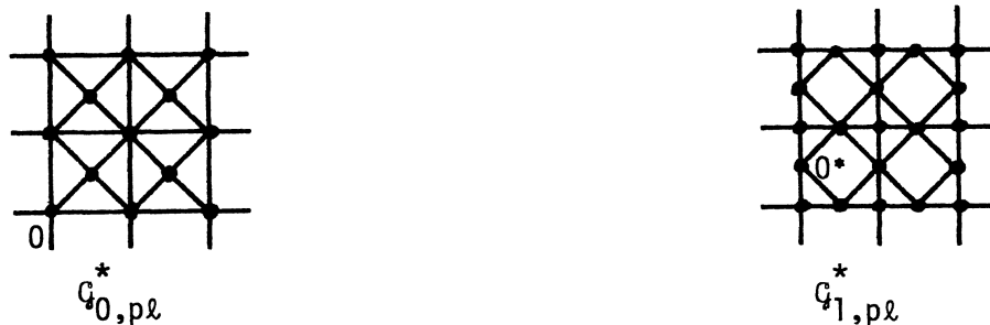
Figure 8.1 Illustration of G_{0,p\ell}^* and G_{1,p\ell}^* . Each black circle represents a vertex. In G_{1,p\ell}^* the origin is marked by * ; it is not a vertex of G_{1,p\ell}^* .
