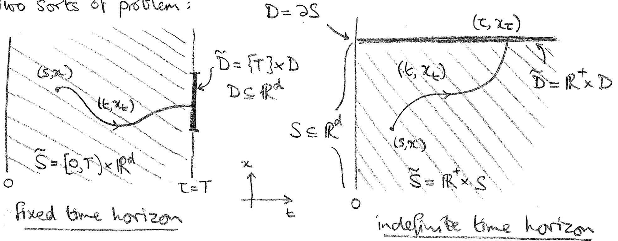
$$\dot{x}_t = b(t, x_t, u_t), \quad x_s = x \quad \text{controlled path}$$
