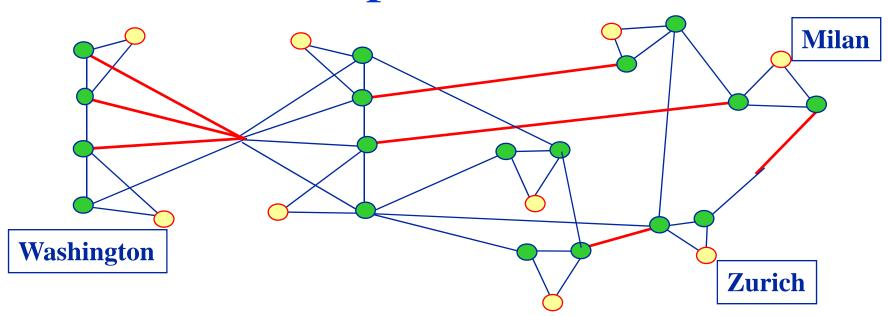
Use  $x_r \propto 1/(T_r \sqrt{p_r})$ to find *T*'s, *p*'s that are consistent with numbers of flows and capacities of resources
