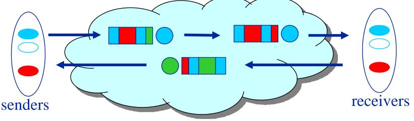
Senders learn (through feedback from receivers) of congestion at queue, and slow down or speed up accordingly. With current TCP, throughput of a flow is proportional to  $\frac{1}{T\sqrt{p}}$
