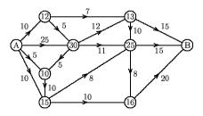
22. By finding a suitable potential on the nodes of the network (i.e., a set of suitable node numbers), show that the flow illustrated below is a minimal-cost circulation. [Each arc is
