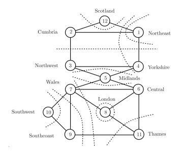
The demand for electricity at node i is  $d_i$ . Node i has  $k_i$  generators, that can generate electricity at costs of  $a_{i1}, \ldots, a_{ik_i}$ , up to amounts  $b_{i1}, \ldots, b_{ik_i}$ . There are n=12 nodes and 351 generators in all. The capacity for transmission from node i to j is  $c_{ij}$  (=  $c_{ji}$ ).
