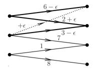
We attempt to increase flow in the dotted arc. Adding an arc to a spanning tree creates a circuit. Increase flow around the circuit until one arc drops out, leaving a new spanning tree. The new solution is
